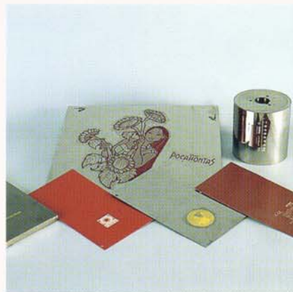
Printing plates Nylon, thin and thick steel printing plates
